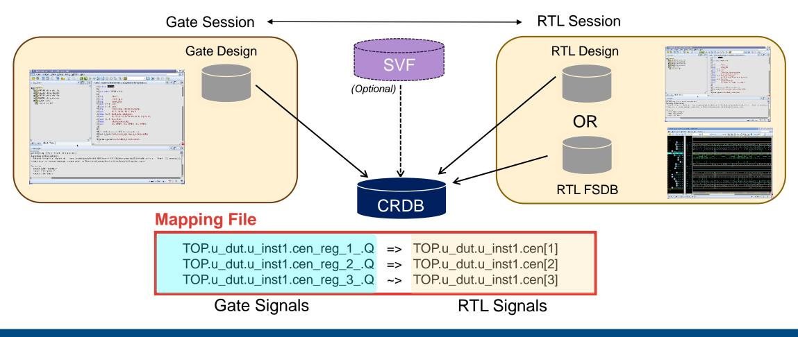
Automatic mapping of signals between RTL and Gate level design
