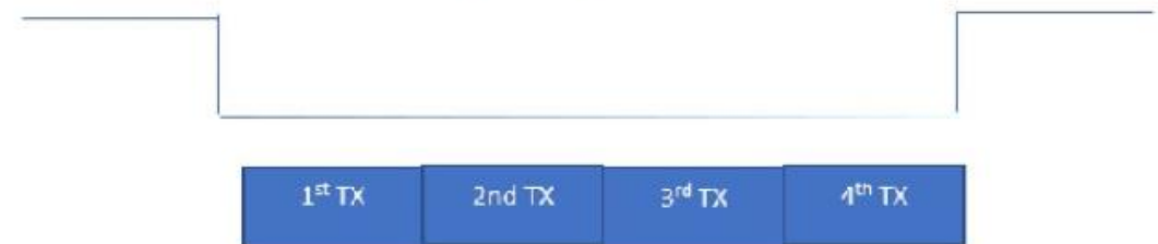
Figure 2-3 Continuous Select Flag Sending 64 Bits of Data
