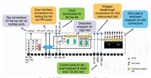
3D DFT components inserted by EDA tool flow.
