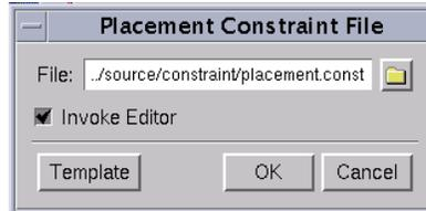
10. Click **OK** to assign a placement constraint for placer related features.
