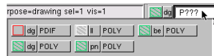
List of layers whose name begins with P and with another three characters.
