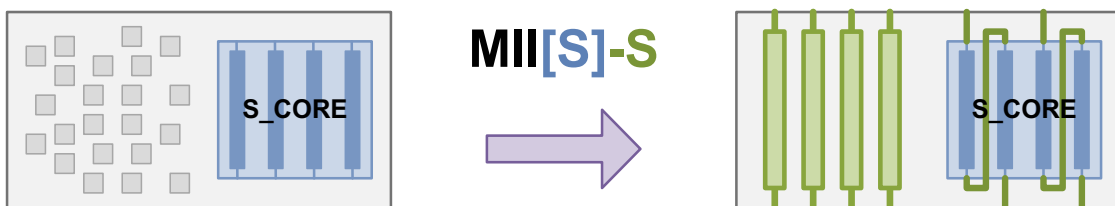
Figure 29-10 Inserting Standard Scan Chains in the MII[C] Flow
