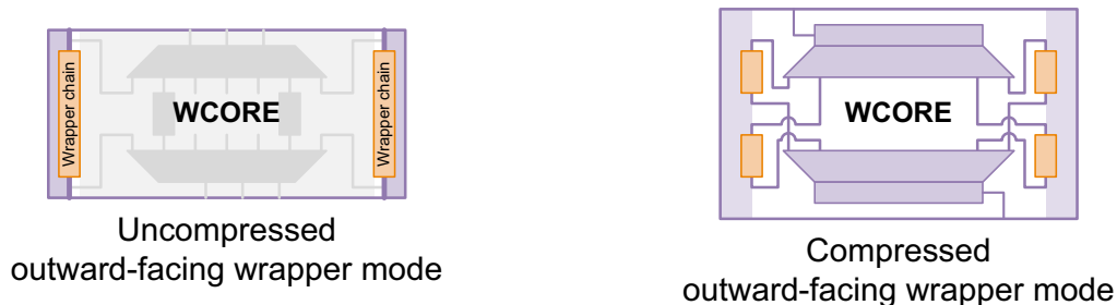
Figure 12-44 Uncompressed and Compressed Outward-Facing (EXTEST) Wrapper Modes
