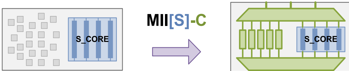
Figure 29-14 Inserting Scan Compression in the MII[C] Flow
