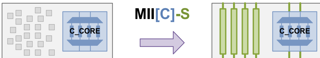
Figure 29-10 Inserting Standard Scan Chains in the MII[C] Flow
