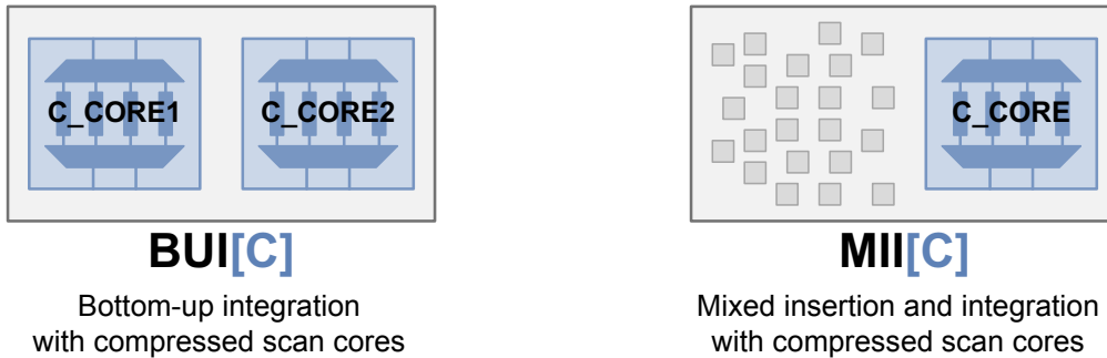
Figure 29-6 [C] Flow Suffix for Existing Compressed Scan Cores
