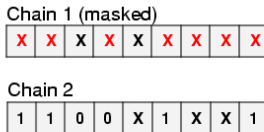
Figure 8-36. Handling of Scan Chain Masking
