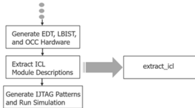
Figure 5-10. Flow for Extracting ICL
