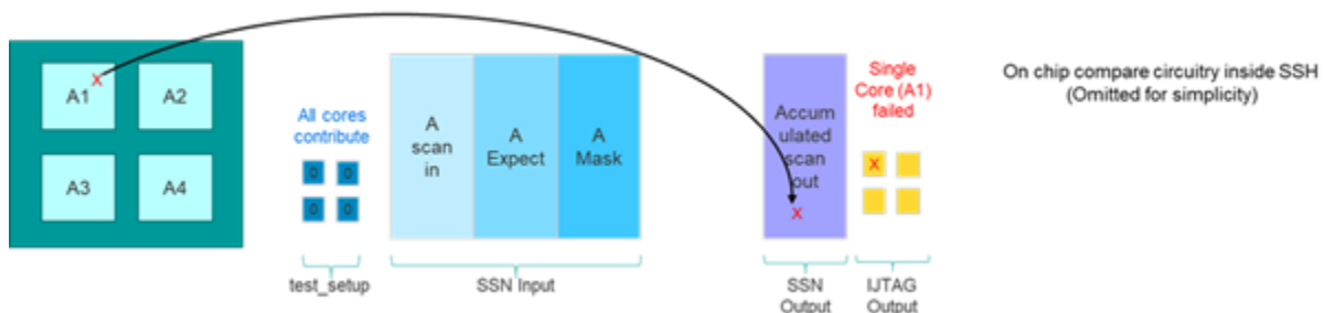
Figure G-2. Single Core Failure Example
