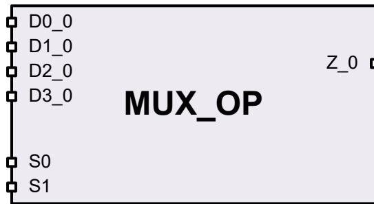
Figure 10 Single-Bit-Wide MUX_OP With Four Selectable Data Inputs
