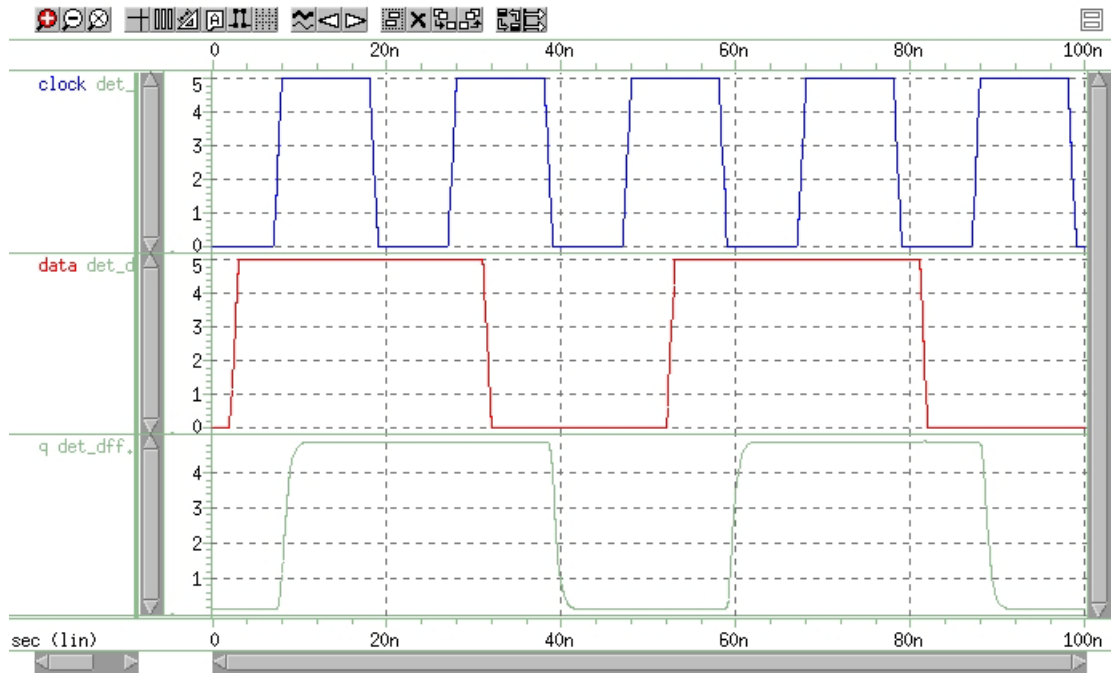
Figure 58 Double Edge Triggered Flip-Flop Response
