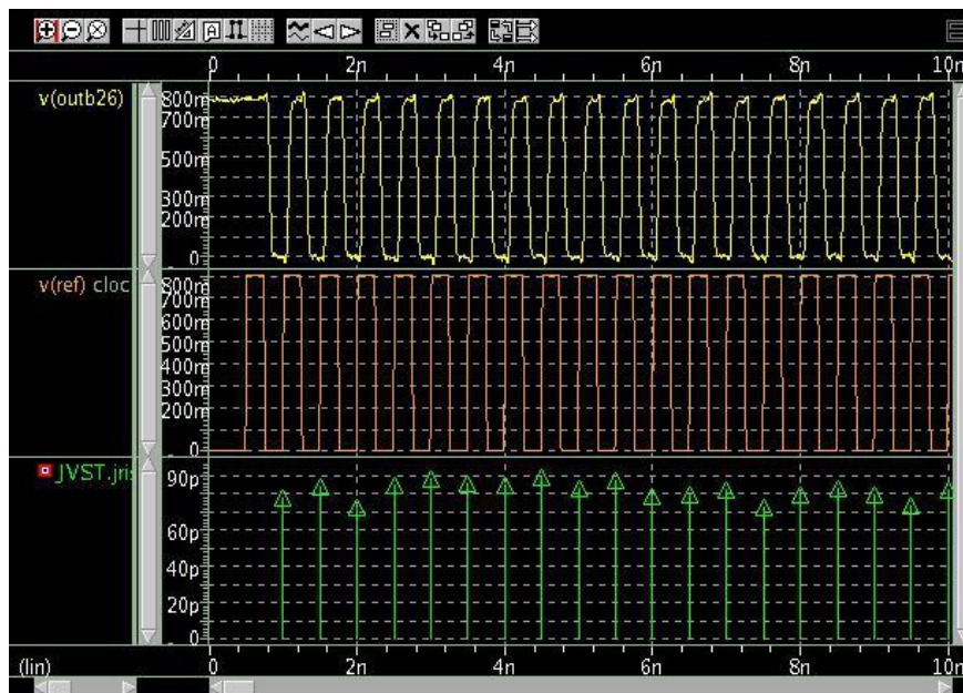
Figure 35 WaveView: Jitter vs. Time measurement to get Timing Interval Error (TIE) Jitter vs. Time. Measurement based on the reference signal
