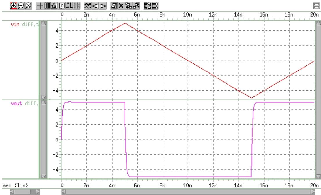
Figure 69 Response of a Differentiator to a Triangle Waveform
