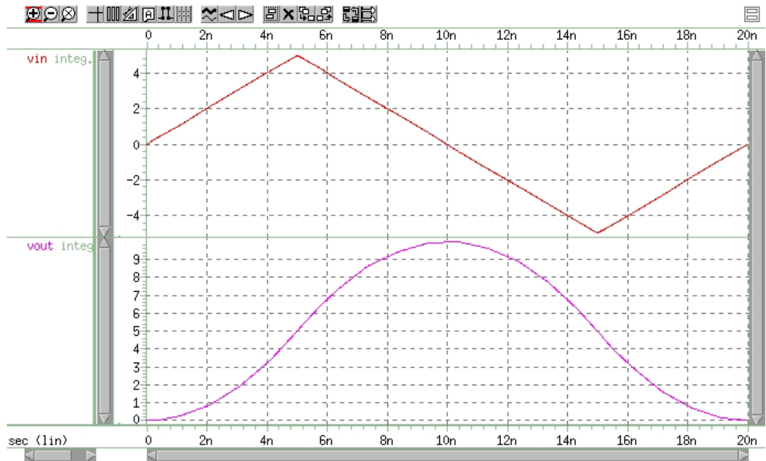
Figure 67 Response of Integrator to a Triangle Waveform
