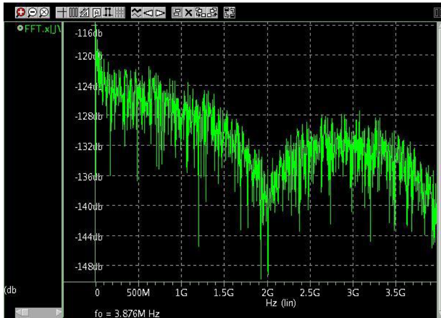
Figure 36 FFT of the TIE Jitter samples show the Jitter Spectrum
