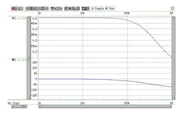
Figure 7 RC Network Node 2 Frequency Response
