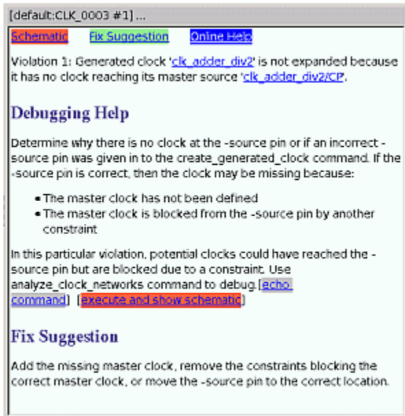
Figure 290 Debugging Help for the CLK_0003 Rule Violation
