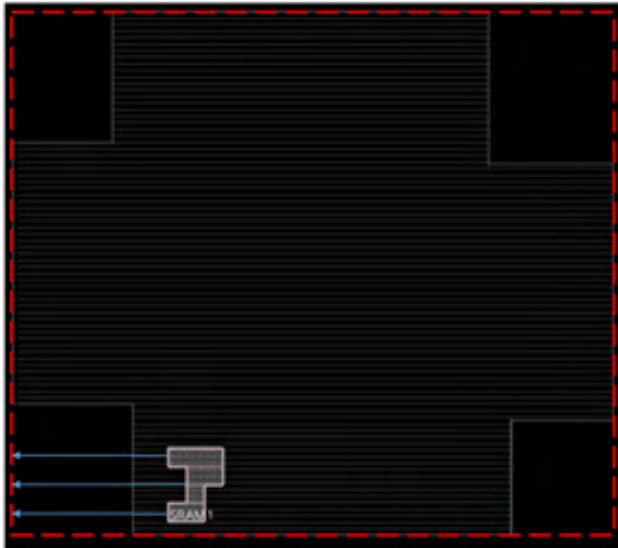
Spacing check between IO pads and other objects (macros and available_sites) in horizontal direction
