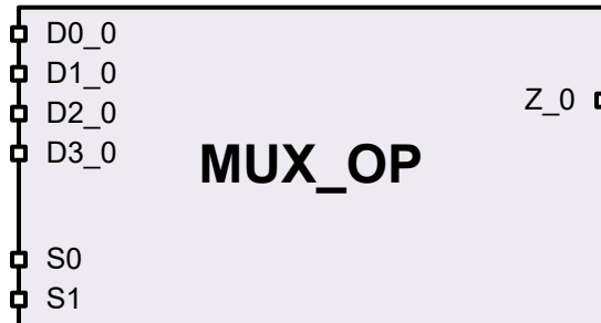
Figure 11 Single-Bit-Wide MUX_OP With Four Selectable Data Inputs
